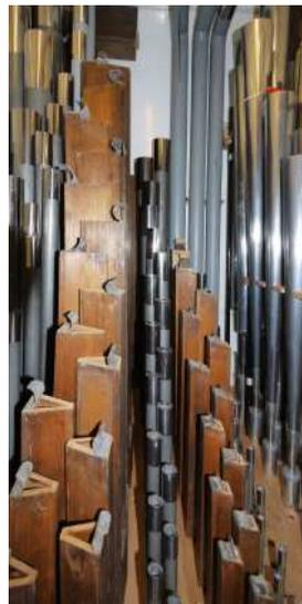
The picture below shows some of the pipes played from the lower keyboard (the Great Organ). The Trumpet pipes on the left are easily recognisable; of 70% tin, they were made by Carl Giesecke in Germany.
