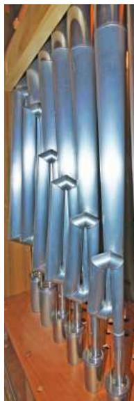
Further ranks of pipes are shown in the picture on the right. Many of these pipes, amounting to approximately half the total number, were transferred from the old organ. Among these are the Hohl Flute pipes which are quite rare, being triangular in shape. All this older pipework was made around 1877. Triangular section flutes had first been introduced by Edmund Schulze a few years earlier, notably in his very large instrument in Doncaster Parish Church. which has five keyboards, or manuals.
